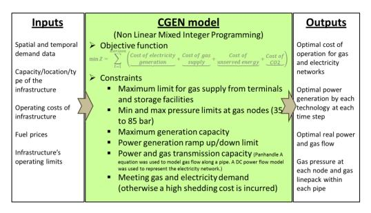
Figure 7: Overview of CGEN model's inputs and outputs
