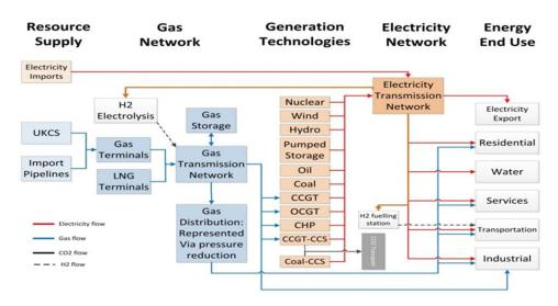
Figure 6: Flow diagram of gas and electricity system considered in CGEN
