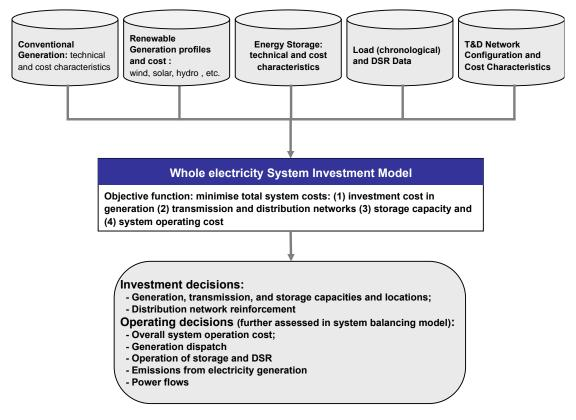
Figure 1: Structure of the WeSIM model
