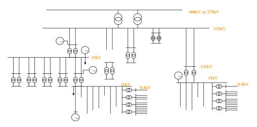
Figure 5: Configuration of representative regional distribution network model
