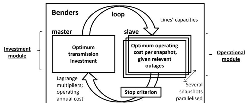
Figure 4: Structure of the DTIM model
