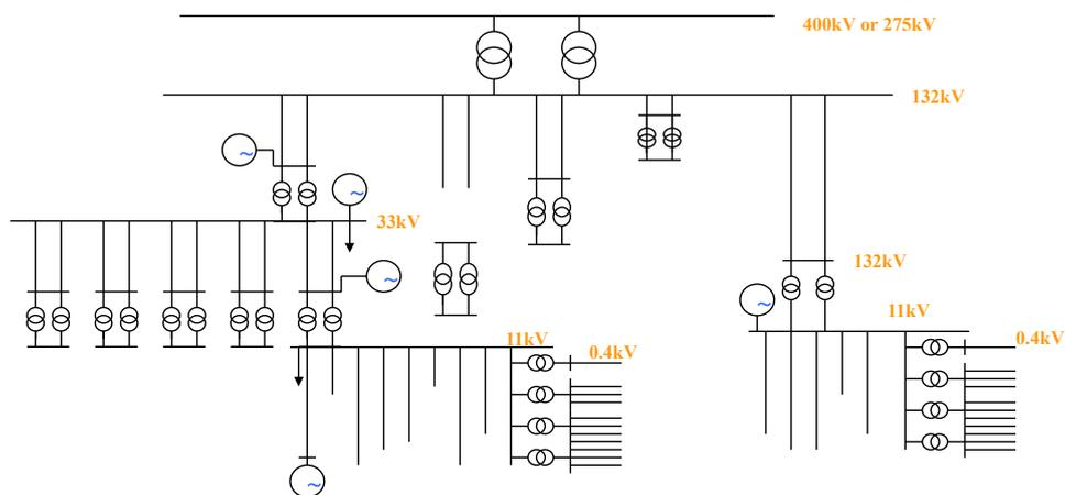
*Figure 5: Configuration of representative regional distribution network model*
