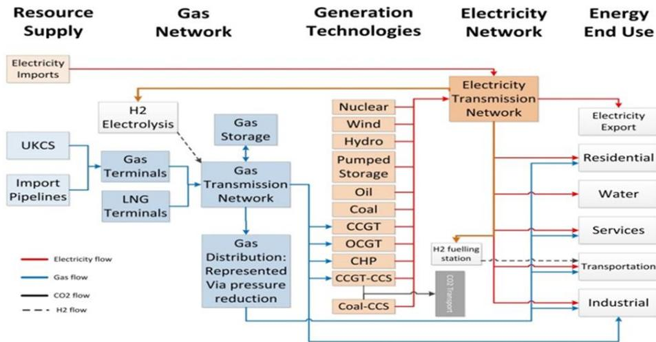
Figure 6: Flow diagram of gas and electricity system considered in CGEN
