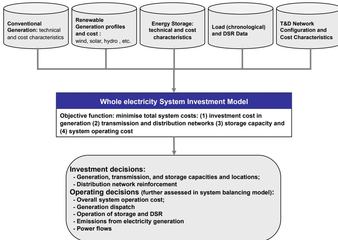
*Figure 1: Structure of the WeSIM model*
