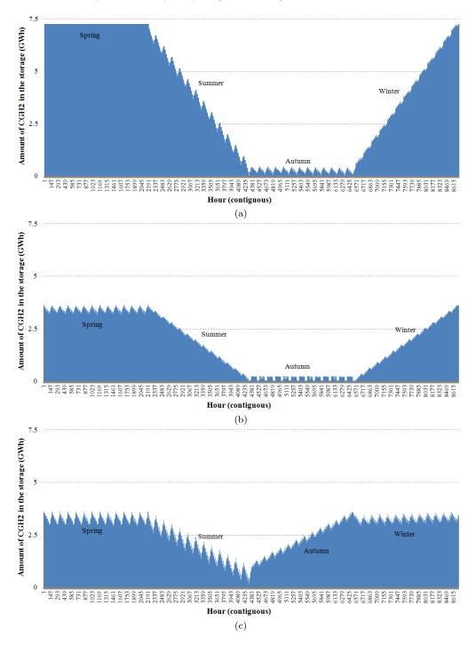
Figure 5 shows the whole-year inventory of hydrogen in storage at different locations in the island.
